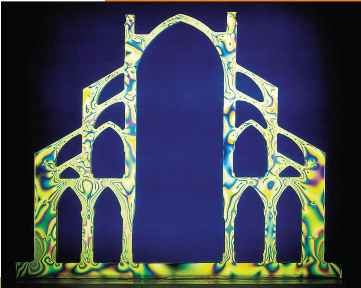
Viewing a plastic model of a structure through crossed pieces of Polaroid filter shows the stress patterns in the structure. This photograph shows a model of the flying buttresses of the Notre Dame cathedral.
