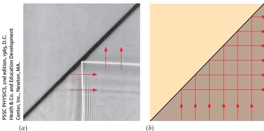
**Figure 19-1** (a) The horizontal white line is a straight water-wave pulse moving toward the top of the picture. The part that has already hit the black barrier is reflected toward the right. (b) The corresponding ray diagram has rays perpendicular to the wave fronts and shows that the angle of reflection is equal to the angle of incidence.
