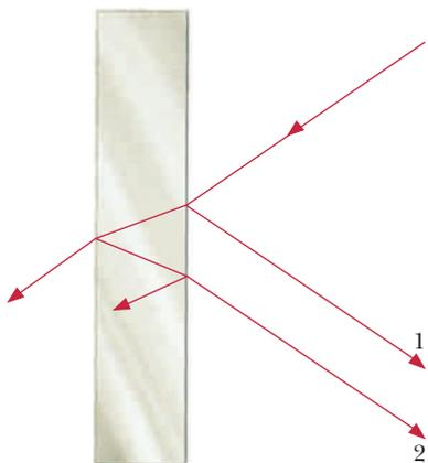
**Figure 19-11** Light incident on a thin film is reflected and transmitted at each surface. Rays 1 and 2 interfere to produce more or less light, depending on the thickness of the film and the wavelength of the light in the film.
