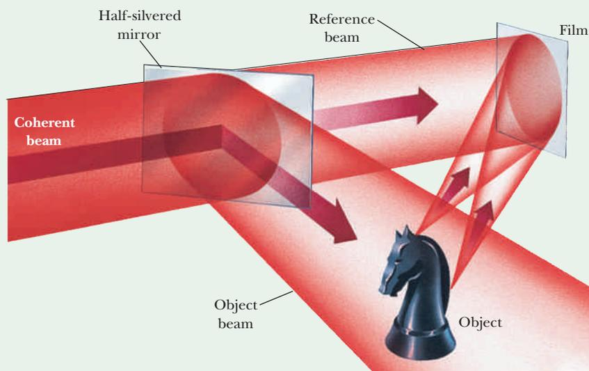
**Figure B** A hologram is viewed by placing it in the reference beam. The light passing through the film produces a virtual image at the location of the original scene.
